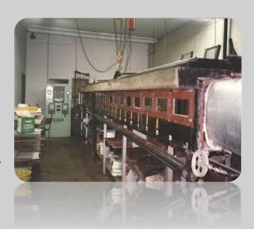
Stainless steel SS304 made Steiner Tunnel Furnace with firebrick interior for resistance to flame impact and good thermal insulation.
